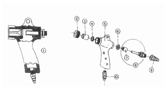
Note: Reference 1, BNP Gun Assembly, does not include the nozzle. Nozzles available for BNP Gun are listed below and must be ordered separately.
